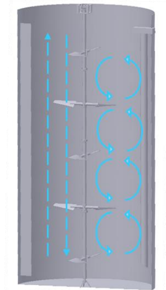
Figure 8. Flow behavior of mixing device of adapted design.
